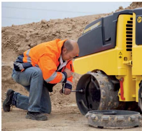
Optional drum extensions change the working width quickly to suit narrower or wider trench widths.
