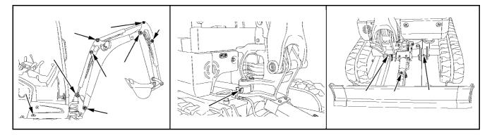
Lubricate all greasing points with grease – see the "Recommended lubricants" section (page 146) – until fresh grease emerges.
