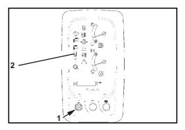
The set flow rate in the right auxiliary port connector and then in the left auxiliary port connector is indicated for few seconds in the display by pressing the display selector switch (1).
