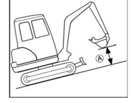
• When driving on gradients, let the bucket slide over the ground if the terrain allows it.
