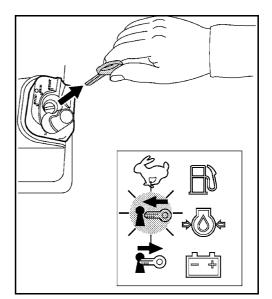
7. After a short moment, the indicator Pull out key blinks. This points out the fact that the black key has been registered for this vehicle.
