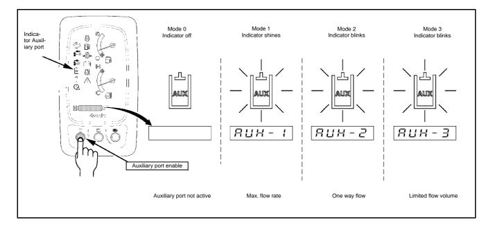
If the auxiliary port is switched on and a mode of operation has been selected, the set flow rate in the right auxiliary port connector and then in the left auxiliary port connector is indicated for few seconds in the display (2) by pressing the display selector switch (1).
