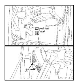
The heater valve (1) in the engine compartment regulates the supply of the heat exchanger with hot water from the cooling cycle.
