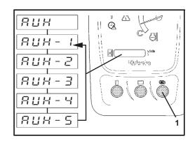
When the selected flow rate is shown on the display, you can use the display selector switch (1) and the menu button (2) to increase or decrease the flow rate.
