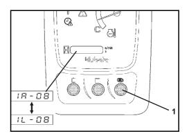
After setting the flow rate for the operating mode selected, you can either switch to the next operating mode or exit the settings screen.
