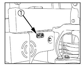
• Operate the excavator and swivel the swivel frame by 90° several times. After greasing, swivel the swivel frame 360° several times to distribute the grease evenly.
